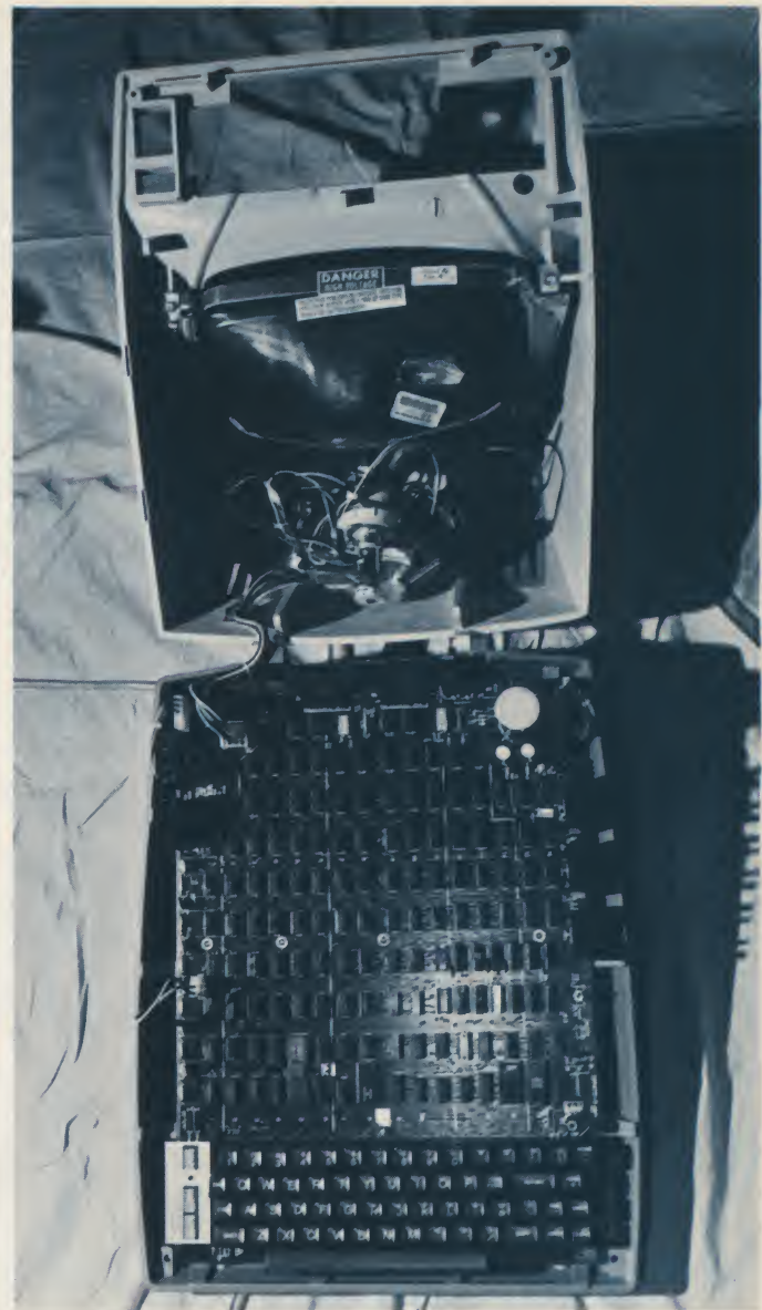
The ADM-3A with clamshell case open to reveal the single major PC board. The keyboard and power supply with heat sinks mount directly onto the main board. Note at the left of the keyboard the option switches, which are accessible with the case closed. The monitor comes preassembled and mounted in the top of the shell, and connection is made to the main board via one plug and cable assembly.
